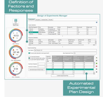
During execution the DoE Manager will minimise raw material usage by automatically moving to the next experiment when steady-state is detected. The sample entry manager streamlines the collection of offline samples by providing automatic timestamping and data alignment. Once an experimental set is complete the subsequent offline results can be entered against the pre-defined experiment and timestamp metadata.
